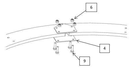
2. Install the  $\frac{1}{4}$ -20 x 2.25" screw (item 10, qty. 4) into Vision Ring Joint Plate. Use 2 unique spacers (items 11 & 12, qty. 1 in each of 4 joints). Attach with nut (item 6, qty. 1 for each plate). **Do not overtighten.**
