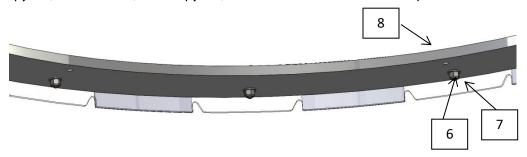
5. Apply 2 cable ties (item 5, qty. 8) at each joint to attach plastic to spacer posts (4 locations)
